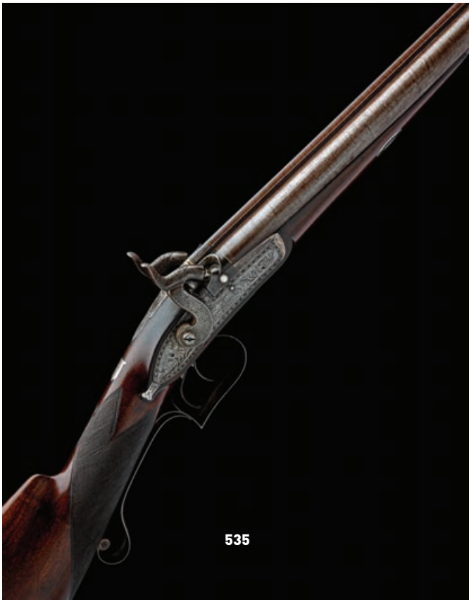
535 AN UNUSUAL 18-BORE PERCUSSION DOUBLE-BARRELLED SPORTING GUN SIGNED CLABROUGH, LINCOLN, no visible serial number , circa 1830, with laminated and browned 30in. barrels, raised concave sighting rib with bead fore-sight, moulded and shallow fenced nipple-wells with twin gold lines to rib-end, platinum plugs, engraved and moulded top-tang, border, scroll and gamescene engraved bar-action locks signed in script 'CLABROUGH LINCOLN, PATENT' and with engraved white metal hook-plates to the bar and tail of each lock, walnut half-stock finely chequered at the wrist and with raised cheek-piece (small filled repair to toe), white metal shield-shaped escutcheon to wrist, engraved iron heel-plate with long triple-staged spur, square-backed and engraved trigger guard bow with shaped grip-safety bar to the lower tang also forming a raised grip, lozenge-headed barrel key with white metal oval escutcheons, engraved ramrod throat and rolled ends to the thimbles, brass mounted ebony ramrod £2,000-3,000
