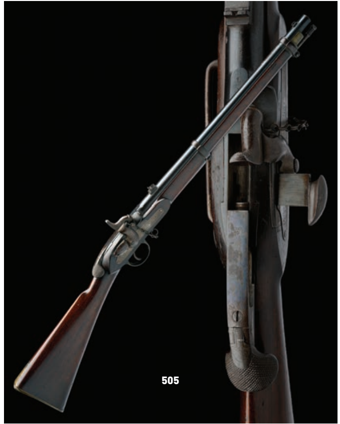
505 A RARE .577 CAPPING BREECH-LOADING PERCUSSION WILSON'S PATENT CARBINE, serial no. A11940 , conforming to British Patent No. 1318, 28th May 1859, with blued 21in. barrel rifled in three grooves, block and blade fore-sight, standing notch rear-sight with two additional folding leaves, the top of breech marked 'WILSON'S PATENT', his trade mark and possibly a South African registration number (neatly applied), unusual sliding bolt with butterfly wing chequered hinged pull-piece and side locking cross bolt, plain lock marked 'TOWER 1869' and stamped with a Queen's crown, walnut full-stock with brass furniture except two iron barrel-bands, saddle-bar, jag-ended ramrod and chained nipple protector, much surface stained finish throughout £800-1,200
