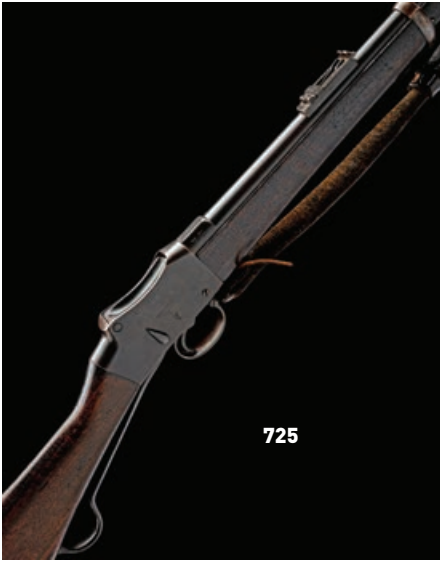
725 A GOOD .577/.450 MARTINI-HENRY MARK IV PATTERN A SIGNED ENFIELD, no visible serial number , dated 1886, with 32 1/2in. sighted barrel with double-row of proof-marks, 'N S / NEP' below back sight for 'Native Service / Nepal', slab-sided receiver marked crown over 'V. R. / ENFIELD / 1886' over lock viewer's mark over offset 'IV / I.', small cocking indicator, falling block action, walnut stock, butt with Madras Arsenal roundel, '11 / 1908' and Nepalese unit script, complete with sling swivets and cleaning rod, black leather SMLE sling, parts with crisp ordnance markings, 49in. overall £500-800
