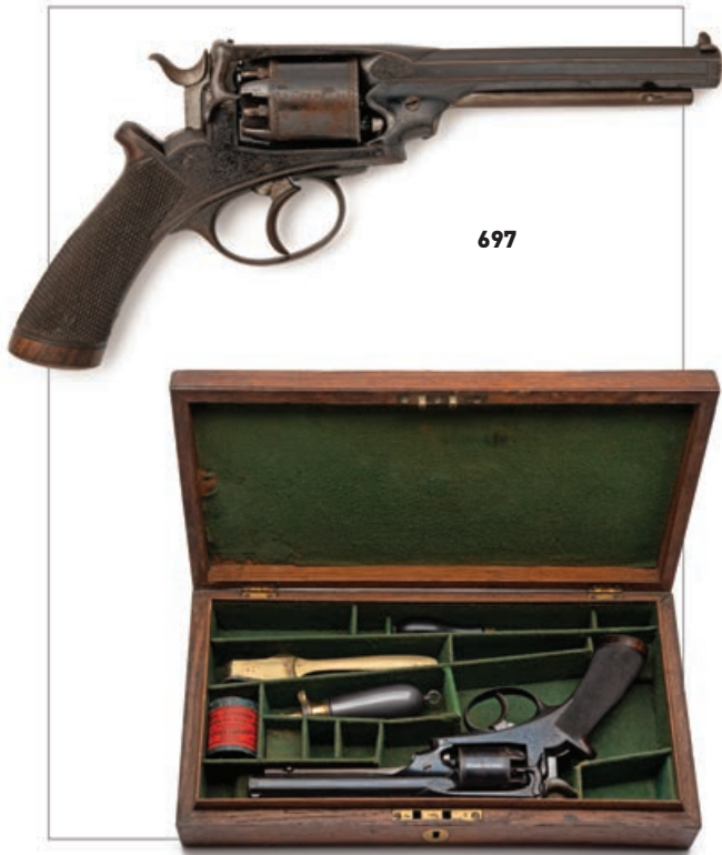
697 A CASED ENGRAVED 54-BORE PERCUSSION DEANE-HARDING PATENT REVOLVER SIGNED DEANE & SON, serial no. 5391 , circa 1860, with blued octagonal 6in. barrel engraved with scrolls at breech, borderlined to the flats and a band at muzzle, the top-strap signed 'DEANE & SON, KING WILLIAM STREET, LONDON BRIDGE' within a border engraved panel, two-piece borderline and scroll engraved blued frame, plain blued cylinder with engraved band to leading edge and broken engraved band to rear, double action mechanism, chequered walnut one-piece saw-handled grip, engraved domed iron butt-cap, guarded trigger and hinged under-barrel rammer, the pistol retaining much of an older London reblue and together with its maker's oak storage case lined and compartmented in green baize and complete with a mould, reproduction flask, cap-tin and nipple-key £1,000-1,500
