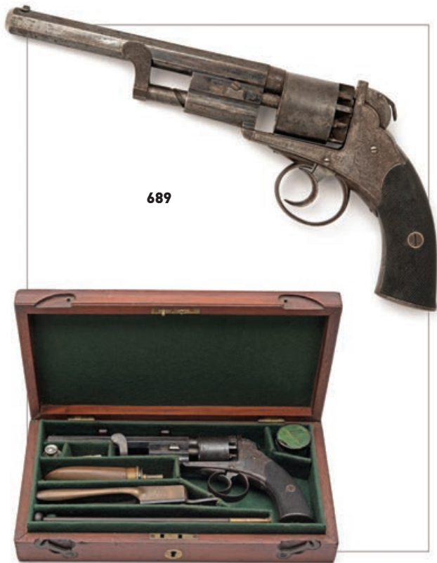
689 A RARE CASED 54-BORE PERCUSSION BENTLEY'S PATENT REVOLVER WITH SCREW RAMMER, serial no. A517 , circa 1855, with blued octagonal 7in. barrel, chamfered muzzle, dove-tailed fore-sight, Bentley's patent screw rammer (conforming to Patent No. 768 of April 4th 1854), wedge barrel key, borderline and scroll engraved open frame with plain five-shot cylinder, standing rear-sight to the top of recoil shield, double action only mechanism, the hammer with Bentley's patent hammer-nose safe (conforming to Patent No. 960 of 1852), finely chequered walnut grips, guarded trigger and in a period mahogany case relined and compartmented and including a mould, loading rod, nipple key, oil bottle and cap-tin, all also period but probably added £1,500-2,000
