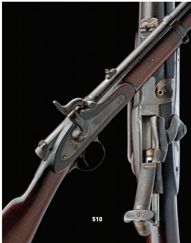
510 A RARE .577 PERCUSSION SWINBURN BREECH-LOADING CARBINE OF BAILEY'S PATENT, patent no. 907 , dated for 1862 and in the style of the British Military Pattern 1861 Cavalry Carbine, with 21 1/2in. iron barrel (finely pitted externally), traces of a stamped inscription 'BAILEY'S PATENT BREECH LOADING CAVALRY * CARBINE' (remainder obscured), shallow block and blade fore-sight, rear-sight of one standing notch and two folding leaves, commercial Birmingham proofs, shaped housing projecting to rear with a lift-up and pull sliding bolt, the top marked 'BAILEY'S PATENT No.907', borderline engraved colour hardened bar-action lock signed 'SWINBURN & SON, PATENT, 1862', walnut full-stock with iron furniture including saddle bar with loose ring to the left side of action and a pan-headed captive iron ramrod, much finish remaining except where noted £1,000-2,000
