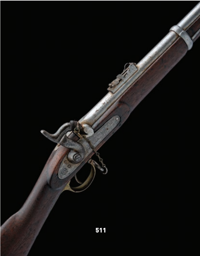
511 A SCARCE .577 PERCUSSION ROBBINS & LAWRENCE WINDSOR PATTERN 1853 ENFIELD RIFLE, no visible serial number , dated for 1856, with refinished in the white 39in. sighted barrel, 'sold out of service' marks at breech, borderline engraved plain lock dated 1856 and signed 'WINDSOR' with a Queen's Crown device at the tail, dark wood full-stock and brass furniture (marked '4L' over '332' over '1.58' on the tang of the heel-plate) with three iron barrel-bands and an iron jag-ended ramrod £400-600
