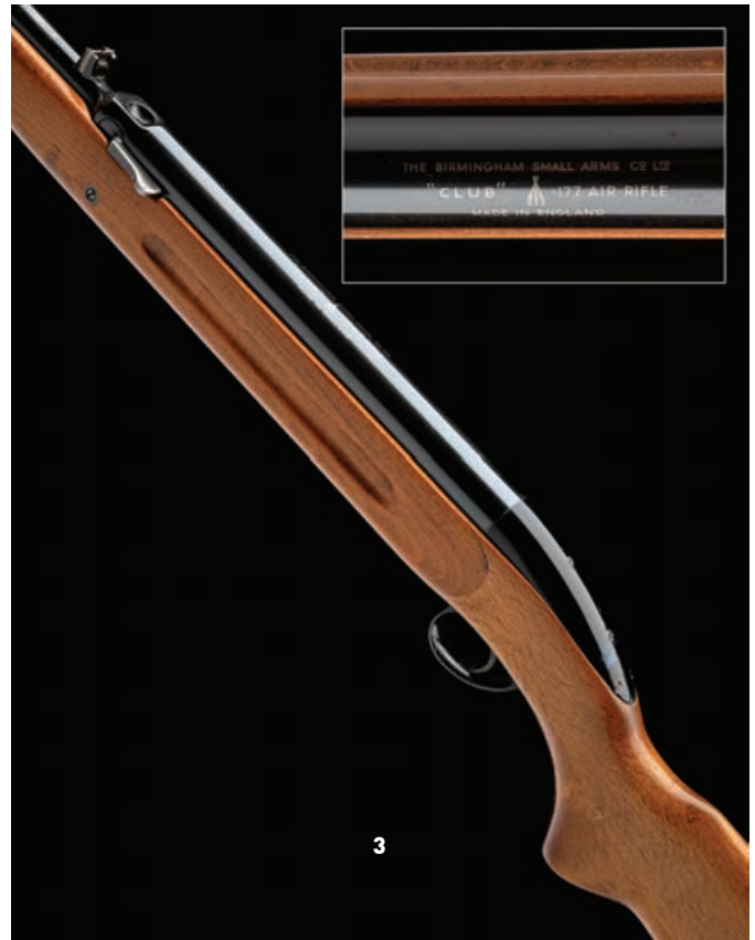
3 A SCARCE .177 BSA CLUB UNDER-LEVER AIR-RIFLE, serial no. EA19608 , for between December 1950 to March 1954, with blued 18in. barrel, ramp fore-sight fitted with a period Parker Hale tunnel sight with interchangeable elements, elevating notch rear-sight, automatic loading tap at breech, plain 9 1/2in. air-chamber, the top of cylinder etched 'THE BIRMINGHAM SMALL ARMS CO LTD' over 'THE CLUB .177 AIR RIFLE' over 'MADE IN ENGLAND' (all etching bright and clear), black stove enamelled trigger unit drilled and tapped for a dedicated folding Parker Hale aperture sight (absent, two of the four holes with keeper-screws), well refinished plain three-piece constructed walnut half-stock with ribbed heel and broad finger-grooves to fore-end, trade mark impressed to left side of butt (rubbed), bakelite stock-bolt cover, concealed under-lever and fitted with sling swivels, the whole generally collector's external condition £400-600
