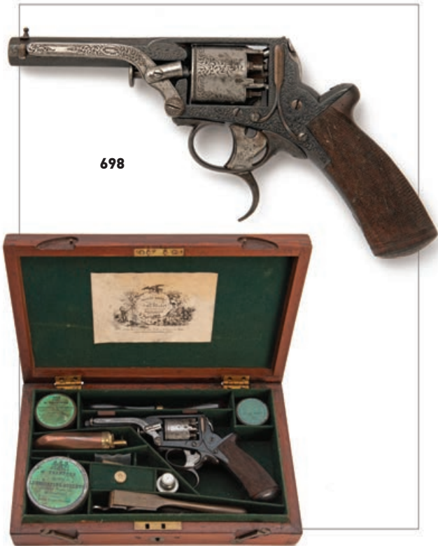
698 A RARE CASED 120-BORE PERCUSSION PRESENTATION GRADE TRANTER PATENT REVOLVER TO ISAAC SMITH, serial no. 13946T , third model circa 1857, with 3 1/2in. octagonal barrel with near full coverage of borderline and scroll engraving, dove-tailed bead fore-sight, shallow notch rear-sight to top of standing breech, the scroll and rope-twist engraved top-strap with central oval panel engraved with the owner's name 'ISAAC SMITH', fully scroll engraved frame, borderline engraved five-shot cylinder with further scroll engraving over each chamber, spurless hammer, inverted 'Y' shaped safe spring, Tranter's patent trigger cocking mechanism, finely chequered walnut butt and scroll engraved rammer, the whole refinished and in its maker's mahogany case lined and compartmented in dark green baize and including a flask, mould, turn-screw, nipple-key and various cap and bullet tins, all contemporary to the revolver, the interior of lid with James Bryce, Edinburgh trade label (lid cracked lengthways) £1,000-1,500
