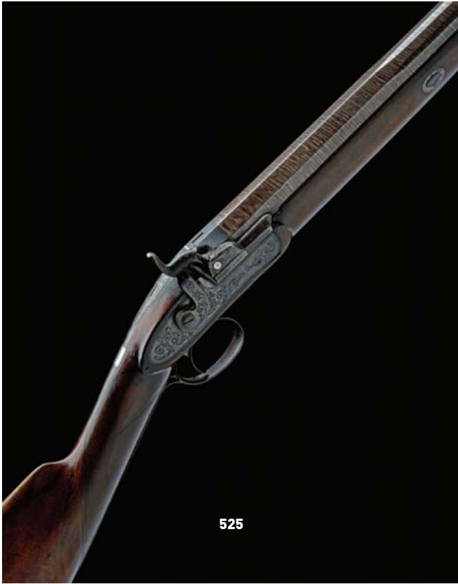
525 AN EARLY 12-BORE PERCUSSION SINGLE-BARRELLED SPORTING GUN BY THOMAS BOSS, LONDON, serial no. 129 , pre-1839, with octagonal to round 32in. laminated browned barrel (later black powder London re-proof), carved girdle at intersection, blued squared patent breech with gold rectangular poinçon to top relief embossed 'THOMAS BOSS PATENT' together with a crown, platinum line and vented plug, borderline and scroll engraved top-tang, border and scroll engraved bar-action lock, signed Thomas Boss 129 on the inside (main spring broken), walnut half-stock with smoothed chequering at wrist, iron furniture except white metal barrel key escutcheons and fore-end tip, ramrod with replacement iron tip (old repairs, and small losses to upper edges of fore-end)
